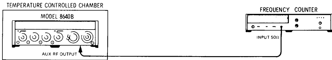
Figure 4-2. Frequency stability vs Temperature Test Setup
